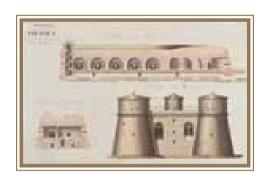
Drawing of the Thüngen redoubt View of the entrance and longitudinal and cross section
